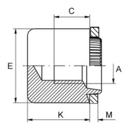
Female thread A = M12Height K = 19.0Min thread length C = 7.0Outer diameter E = 25.0Plate thickness = 0.9 to 1.0
